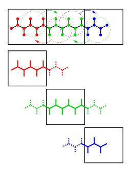
Figure 3.14: Example of the parallel setup of P-LINCS with one molecule split over three domain decomposition cells, using a matrix expansion order of 3. The top part shows which atom coordinates need to be communicated to which cells. The bottom parts show the local constraints (solid) and the non-local constraints (dashed) for each of the three cells.
