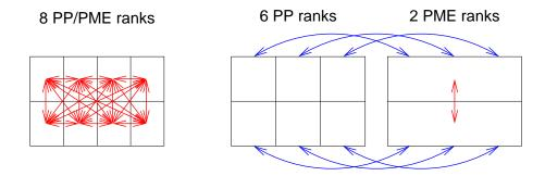
Figure 3.15: Example of 8 ranks without (left) and with (right) MPMD. The PME communication (red arrows) is much higher on the left than on the right. For MPMD additional PP - PME coordinate and force communication (blue arrows) is required, but the total communication complexity is lower.
