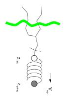
Figure 6.1: Schematic picture of pulling a lipid out of a lipid bilayer with umbrella pulling.  $V_{rup}$  is the velocity at which the spring is retracted,  $Z_{link}$  is the atom to which the spring is attached and  $Z_{spring}$  is the location of the spring.
