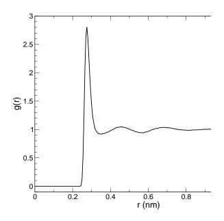
Figure 8.3:  $g_{OO}(r)$  for Oxygen-Oxygen of SPC-water.
