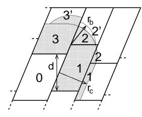
Figure 3.13: The zones to communicate to the rank of zone 0, see the text for details.  $r_c$  and  $r_b$  are the non-bonded and bonded cut-off radii respectively, d is an example of a distance between following, staggered boundaries of cells.
