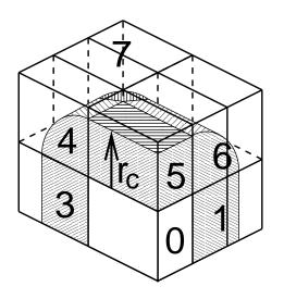
Figure 3.12: A non-staggered domain decomposition grid of  $3 \times 2 \times 2$  cells. Coordinates in zones 1 to 7 are communicated to the corner cell that has its home particles in zone 0.  $r_c$  is the cut-off radius.
