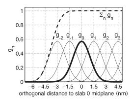
Figure 6.5: Gaussian functions  $g_n$  centered at  $n \Delta x$  for a slab distance  $\Delta x = 1.5$  nm and  $n \ge -2$ . Gaussian function  $g_0$  is highlighted in bold; the dashed line depicts the sum of the shown Gaussian functions.
