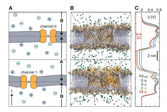
Figure 6.6: Typical double-membrane setup for CompEL simulations (A, B). Plot (C) shows the potential difference  $\Delta U$  resulting from the selected charge imbalance  $\Delta q_{ref}$  between the compartments.
