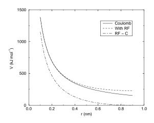
Figure 4.3: The Coulomb interaction (for particles with equal signed charge) with and without reaction field. In the latter case  $\varepsilon_r$  was 1,  $\varepsilon_{rf}$  was 78, and  $r_c$  was 0.9 nm. The dot-dashed line is the same as the dashed line, except for a constant.
