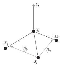
Figure 4.20: The new 4fdn virtual site construction, which is stable even when all constructing atoms are in the same plane.
