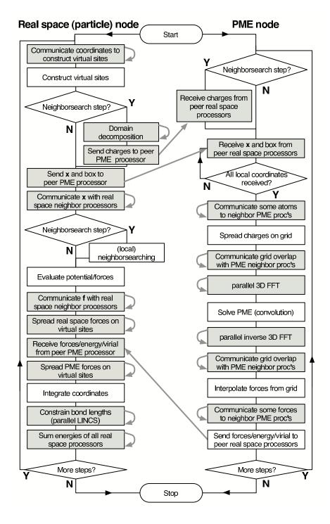
Figure 3.16: Flow chart showing the algorithms and communication (arrows) for a standard MD simulation with virtual sites, constraints and separate PME-mesh ranks.
