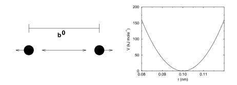
Figure 4.5: Principle of bond stretching (left), and the bond stretching potential (right).
