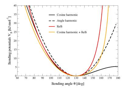
Figure 4.8: Bending angle potentials: cosine harmonic (solid black line), angle harmonic (dashed black line) and restricted bending (red) with the same bending constant  $k_{\theta} = 85$  kJ mol<sup>-1</sup> and equilibrium angle  $\theta_0 = 130^{\circ}$ . The orange line represents the sum of a cosine harmonic (k = 50 kJ mol<sup>-1</sup>) with a restricted bending (k = 25 kJ mol<sup>-1</sup>) potential, both with  $\theta_0 = 130^{\circ}$ .
