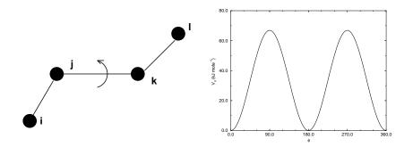
Figure 4.11: Principle of proper dihedral angle (left, in *trans* form) and the dihedral angle potential (right).
