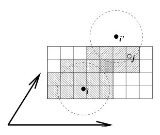
Figure 3.6: Grid search in two dimensions. The arrows are the box vectors.
