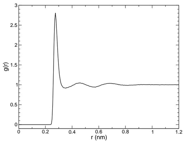
Figure 8.3:  $g_{OO}(r)$  for Oxygen-Oxygen of SPC-water.
