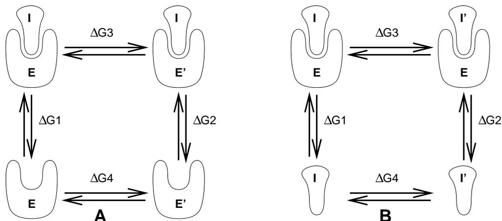
Figure 3.11: Free energy cycles. **A:** to calculate  $\Delta G_{12}$ , the free energy difference between the binding of inhibitor **I** to enzymes **E** respectively **E'**. **B:** to calculate  $\Delta G_{12}$ , the free energy difference for binding of inhibitors **I** respectively **I'** to enzyme **E**.
