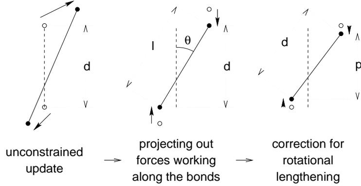
Figure 3.10: The three position updates needed for one time step. The dashed line is the old bond of length  $d$ , the solid lines are the new bonds.  $l = d \cos \theta$  and  $p = (2d^2 - l^2)^{\frac{1}{2}}$ .
