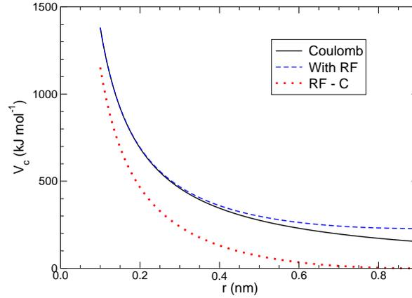
Figure 4.3: The Coulomb interaction (for particles with equal signed charge) with and without reaction field. In the latter case  $\epsilon_r$  was 1,  $\epsilon_{rf}$  was 78, and  $r_c$  was 0.9 nm. The dot-dashed line is the same as the dashed line, except for a constant.
