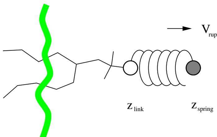
Figure 6.1: Schematic picture of pulling a lipid out of a lipid bilayer with umbrella pulling.  $V_{rup}$  is the velocity at which the spring is retracted,  $Z_{link}$  is the atom to which the spring is attached and  $Z_{spring}$  is the location of the spring.
