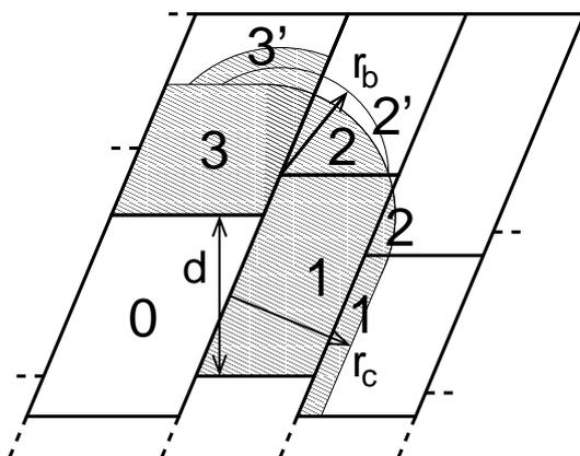
Figure 3.13: The zones to communicate to the processor of zone 0, see the text for details.  $r_c$  and  $r_b$  are the non-bonded and bonded cut-off radii respectively,  $d$  is an example of a distance between following, staggered boundaries of cells.
