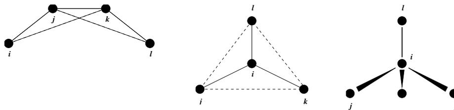
Figure 4.8: Principle of improper dihedral angles. Out of plane bending for rings (left), substituents of rings (middle), out of tetrahedral (right). The improper dihedral angle  $\xi$  is defined as the angle between planes (i,j,k) and (j,k,l) in all cases.
