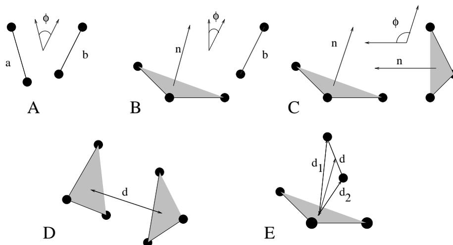
Figure 8.6: Options of `g_sgangle`: A. Angle between 2 vectors. B. Angle between a vector and the normal of a plane. C. Angle between two planes. D. Distance between the geometrical centers of 2 planes. E. Distances between a vector and the center of a plane.
