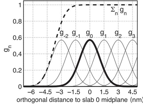
Figure 6.5: Gaussian functions  $g_n$  centered at  $n \Delta x$  for a slab distance  $\Delta x = 1.5$  nm and  $n \geq -2$ . Gaussian function  $g_0$  is highlighted in bold; the dashed line depicts the sum of the shown Gaussian functions.
